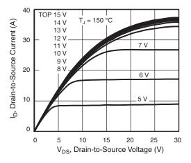
Fig. 2 - Typical Output Characteristics
