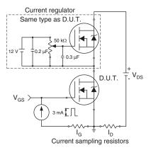
Fig. 17 - Gate Charge Test Circuit
