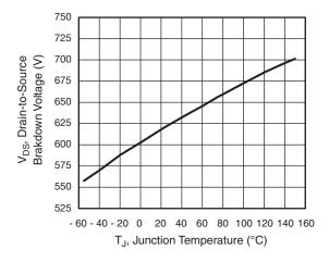
Fig. 10 - Temperature vs. Drain-to-Source Voltage
