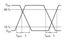
Fig. 13 - Switching Time Waveforms
