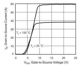
Fig. 3 - Typical Transfer Characteristics
