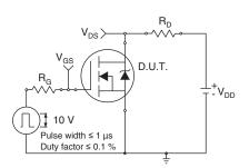
Fig. 12 - Switching Time Test Circuit
