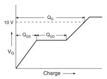
Fig. 16 - Basic Gate Charge Waveform
