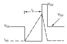
Fig. 15 - Unclamped Inductive Waveforms
