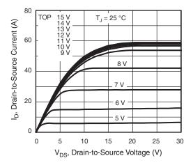
Fig. 1 - Typical Output Characteristics
