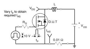
Fig. 14 - Unclamped Inductive Test Circuit
